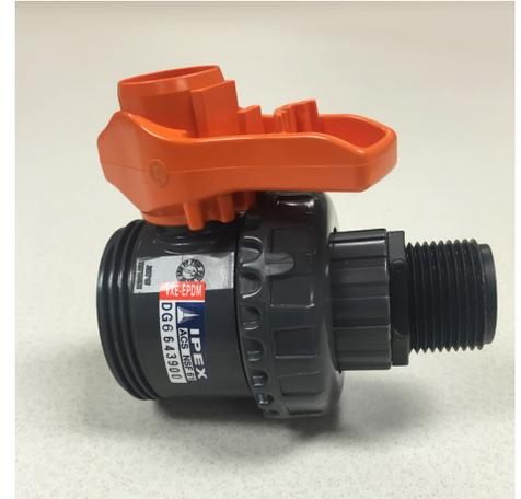
Place upside down handle on true-union ball valve and line up notches to use as a wrench to tighten or loosen fittings.
