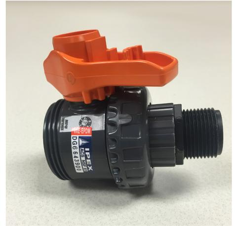
Place upside down handle on tru-union ball valve and line up notches to use as a wrench to tighten or loosen fittings.
