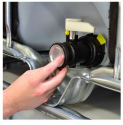
Remove the tamper evident NSF seal from the tote valve.
