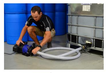
Attach other end of hose to 1.5" pumping system and finish setting up circulation system.
